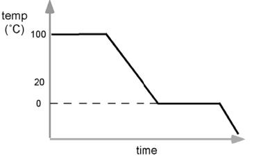
In our energy flow diagram we would show energy leaving the system via heating. On the plateaus, the system was giving up  $E_{ph}$  as the phase changed. On the declines, the temperature was changing and the system lost  $E_{th}$ .
