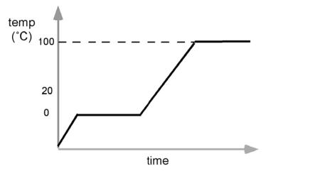
In our energy flow diagram we would show energy entering the system via heating during this series of changes. On the plateaus, the phase was changing and the system was storing  $E_{ph}$ . On the inclines, the temperature was changing and the system stored  $E_{th}$ .
